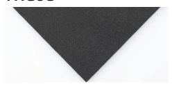
This material is a closed-cell flame retardant and self-extingushing grade. It fully complies with UL94-HF1 and FMVSS302 fire safety standards. It has a working temperature range from -40°C to +80°C. We supply this material in densities ranging from 130 to 170 kg/m³ in thicknesses from 1mm to 40mm as standard.
